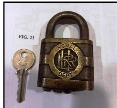
(Right) This is a brass Signal Department lock with cast lettering for "LIRR" intertwined on the front of lock and "Yale" cast on the back of lock. This lock takes a flat steel key (unmarked) and was possibly used to lock a box containing a staff at one end of a bridge (double track into single track across the bridge) allowing the holder of the staff to proceed. Circa 1920's.
