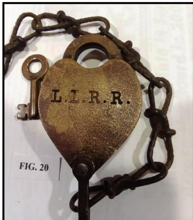
(Left) This is a brass heart shaped Signal Department lock marked "Wilson Bohannon Brooklyn, N. Y." the key is of the center turn type and it is attached to a length of chain. On the reverse in larger letters "L. I. R. R." is engraved. This lock takes a small brass key with "LIRR" and "Employee No. 2519". Circa 1920's.
