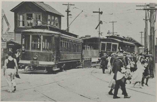
Ocean Electric No. 30 and No. 7 at Beach 84th St. Hammels in 1922. Note both trolley pole and shoe (F. Goldsmith)
