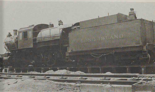
#14, a 4-6-0 dual service Camelback, Baldwin 1902, series G-54B. (Holman Collection) (Top) #6, a 4-6-0 dual service Camelback, Baldwin 1901, series G-54B. (Bottom)
