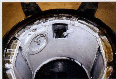
Headlight barrel interior with light gray paint, showing access port and spare bulb box.
