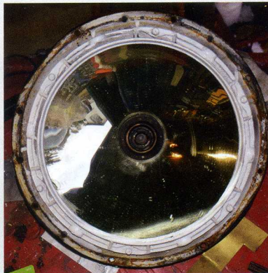
Polished glass reflector, showing metal retaining ring.
