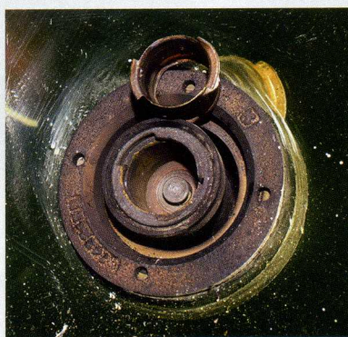
Brass bayonet style ring to fit over threaded bulb, before inserting into the receptacle (shown).
