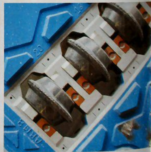
These are the cutting heads of a tunnel boring machine. TBMs are specialized to deal with hard rock, like in Manhattan, or a mix of rock and soft soils, like in Queens.
