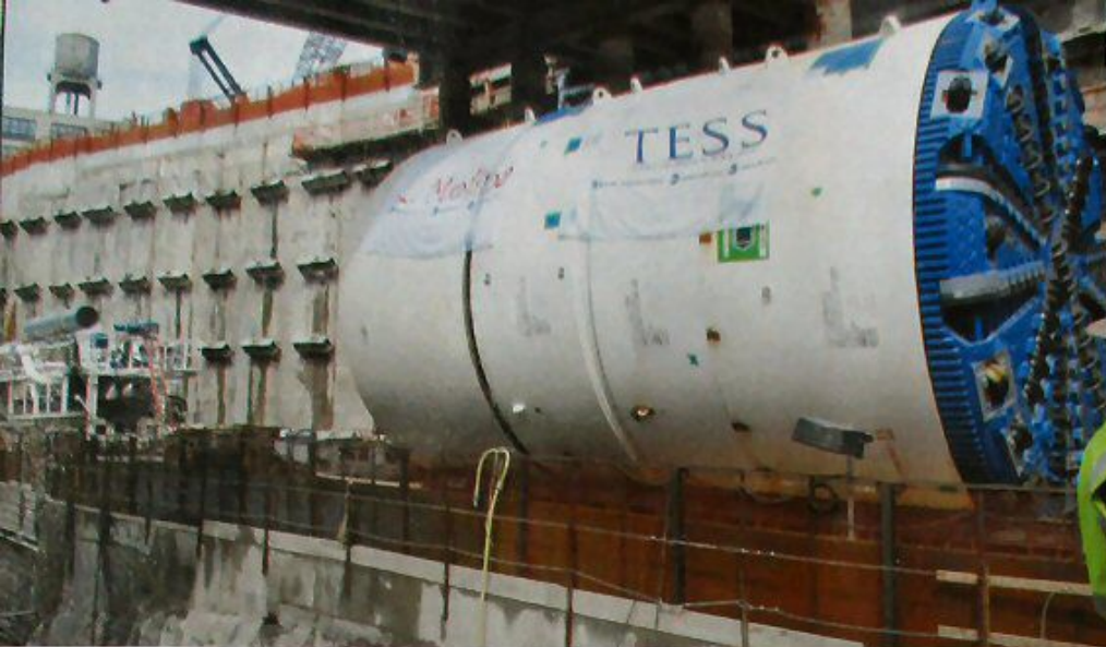
This is one of two tunnel boring machines that cut under Sunnyside Yard in Queens, N.Y. Two more, from Italy, bored under Park Avenue in Manhattan.
