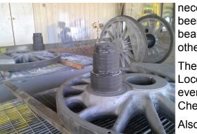
necessary. Once the drive wheels have been renewed, work will continue on the bearing boxes, drive rods, pins and other components of the running gear.
