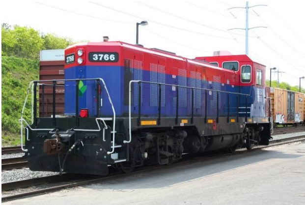
The RSSX 3766, a gen-set locomotive built on a frame from a T&NO locomotive. This locomotive is leased from Rail Switching Services by the BRT.
