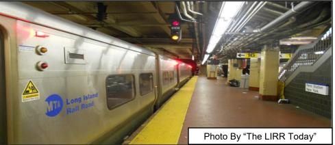
engineer has the authority to proceed. HOWEVER, at Penn Station, there are situations where the leading end of the train may be past the initial signal required for the movement. How does the engineer know the signal to proceed is displayed? The engineer has to be told by the Conductor, or granted permission by the Dispatcher.
