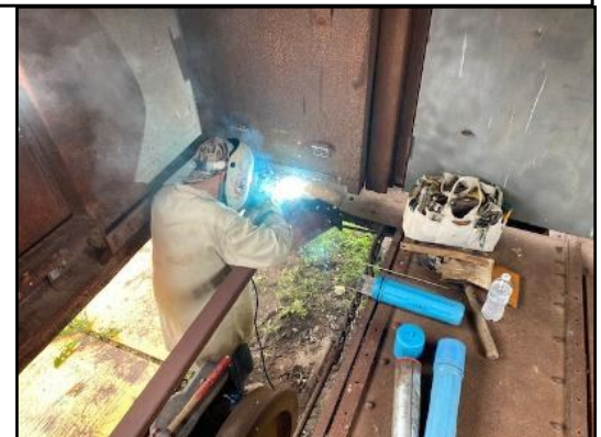
Ping Pong Coach work included the repair of the window ledges and installation of additional floor supports.
