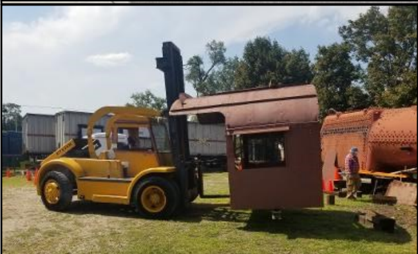
Steam Locomotive #35 work included the final preparation work before painting of the cab and the installation of new studs on the boiler.
