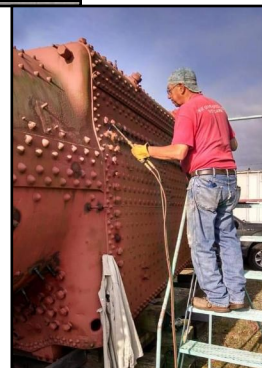
Steam Locomotive #35 work included the final preparation work before painting of the cab and the installation of new studs on the boiler.
