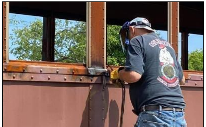
Ping Pong Coach work included the repair of the window ledges and installation of additional floor supports.
