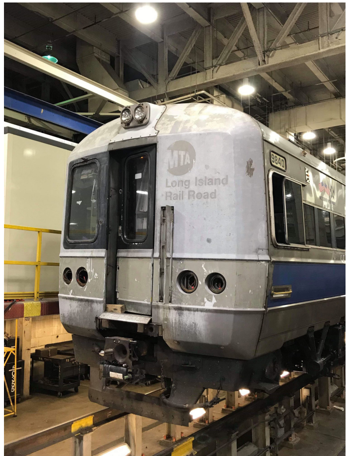
An M-3 being prepped for repainting
