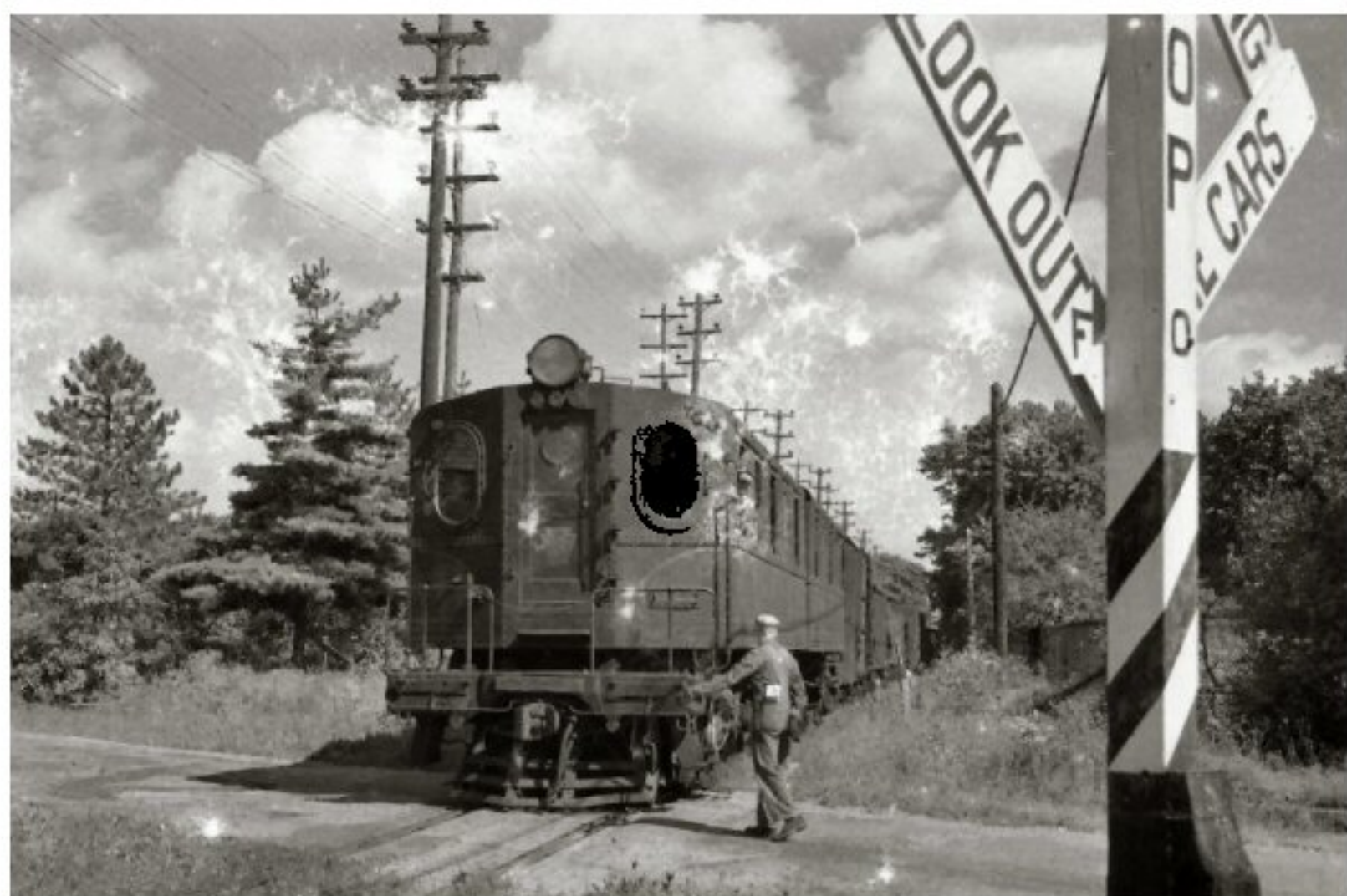
DD1 #358 pulling freight westbound of West Hempstead station. The freight brakeman had to flag each crossing. 9/28/1947 Archive: Dave Keller
