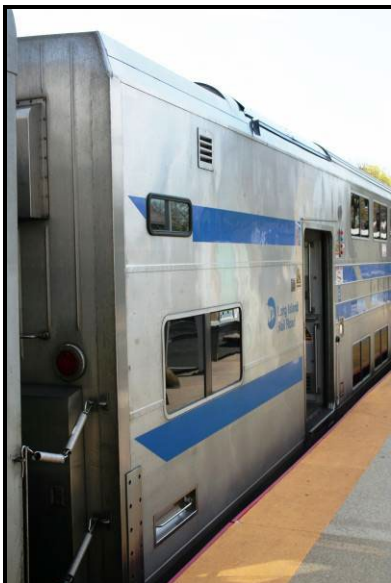
The 'B' end of the C3-C and C3-T/T coaches are blank, the C3-T has a window at this position. Car 4054 at Roslyn on April 14, 2012.
