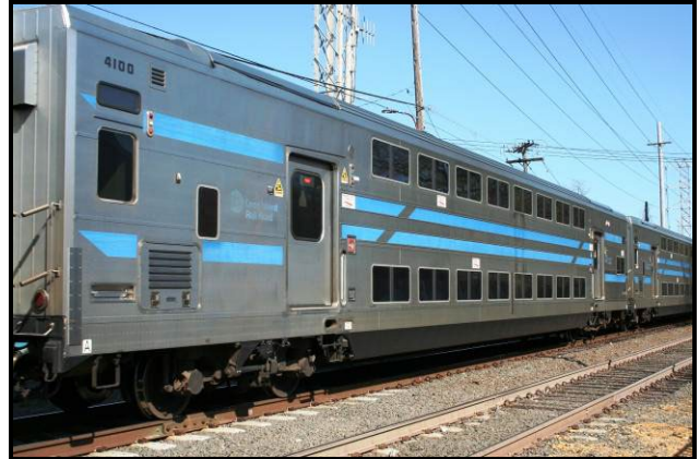
C-3T passenger coach 4100 in the consist of Train 415 at Roslyn. This is an eighty-five foot long bi-level passenger coach seating 143 passengers, and weights seventy-one tons. There are sixty-seven of these cars with even numbers only from 4002 to 4134; they were built by Kawasaki Heavy Industries. These cars have seating with a window at the far end in lieu of the toilet compartment.
