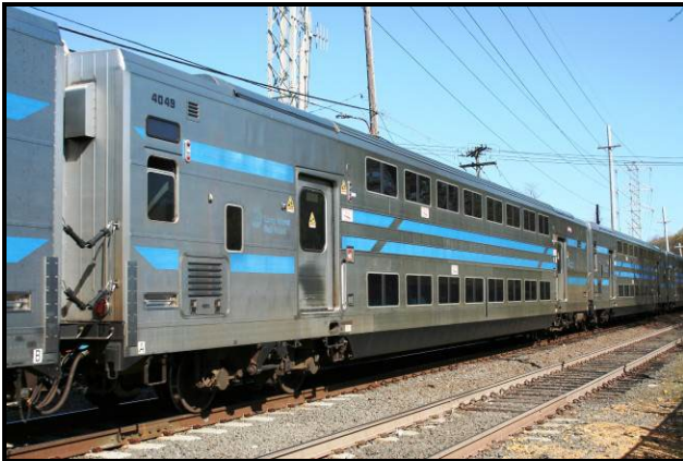
C-31/T passenger coach 4049 in the consist of Train 415 at Roslyn. This is an eighty-five foot long bi-level passenger coach seating 137 passengers, has a toilet facility (at the far end), and weights seventy-three tons. There are forty-four of these cars with odd numbers only from 4001 to 4087; they were built by Kawasaki Heavy Industries and all went into revenue service during 1997.
