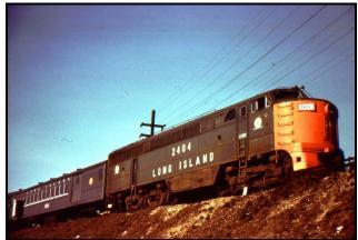
(Left) In September 1951, four additional passenger cab locomotives came to the island. They were CPA04-5 2400 horsepower units numbered 2401 to 2404. They usually worked the Port Jefferson trains or the heavier trans to Montauk. Again, they were traded in to Alco Products in the first quarter of 1964 on the first C420 order. The 2404 is seen here in a William Rugen photograph, probably in the Richmond Hill yard area.
