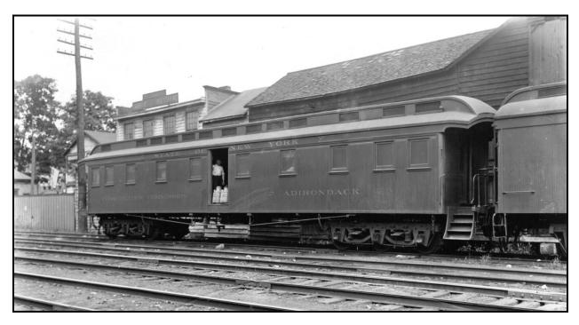
A further Ray Breyer scan was a diagram that allowed for some basic measurements and proportions to be laid out. While not scaled a few possibly "known" measurements were assumed; overall width of 10' more or less (as being a common dimension used in the 19th Century design and build of wooden passenger car types) and a six-wheel truck wheelbase of 10' 6" to 10' 8" (not so very much difference in HO Scale).
