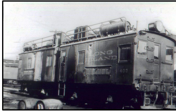
The 403A and 403B in Morris Park between January 1928 and December 1929, note the leaks on the carbody side from the roof top radiators. Undated image from the collection of Paul Garde.
